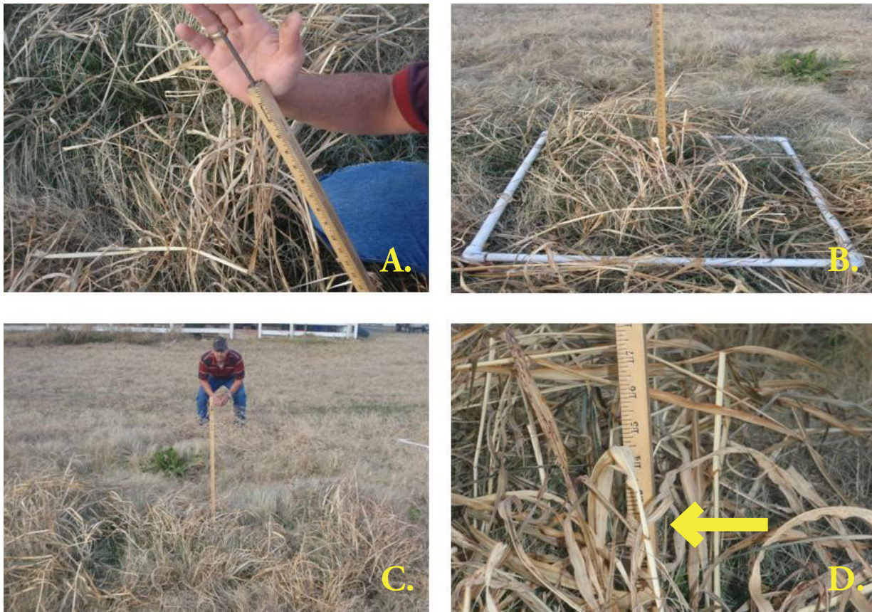
Figure 1. Steps in use of yard stick as prescribed by Robel et al. (1970) to estimate plant biomass in short grass prairies of Texas. Example of yard stick with modified nail tip (A), Step 1 – placement of yard stick in sample plot (B), Step 2 – estimating visual obstruction index from a distance of 13 feet (C), and Step 3 – recording of visual obstruction index, lowest observation point illustrated with arrow (D).
